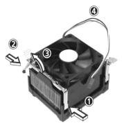
4 Connect the 3-pin fan/thermal cable to the system board. Refer to section "System board layout" on page 23 for the location of the fan/thermal connectors.
